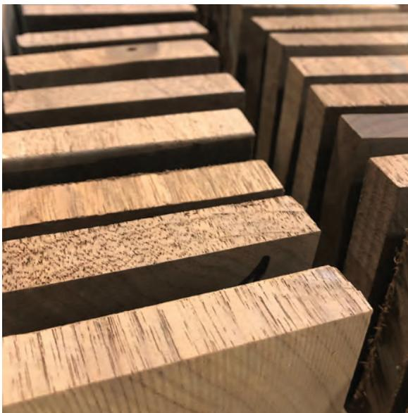
2. Due to the orientation of the grain, end-grain flooring tends to equilibrate at a relatively fast rate (depending on thickness and species) as compared to other solid sawn
