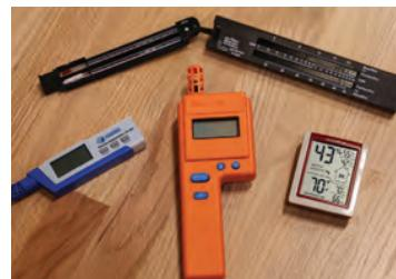
oftentimes properties like absolute humidity and dew point as well. Many of today's thermo-hygrometers are wireless, have data logging, and even have remote capabilities.
