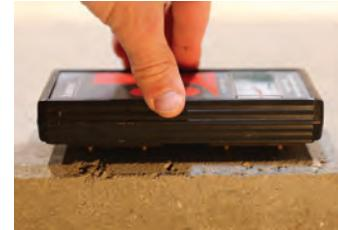
gypsum cement, and other floor slabs and screeds. It is a nondestructive testing method. These tests should be used to evaluate the surface of the concrete and to determine where to place other quantifiable tests. These tests provide useful information, but should not be used on their own to determine whether a floor should or should not be installed unless otherwise directed by the flooring manufacturer.
